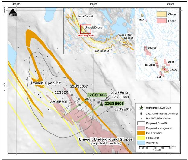
Figure 2.0: Goose Property plan map showing 2022 drilling, targeting the Umwelt Deposit.
